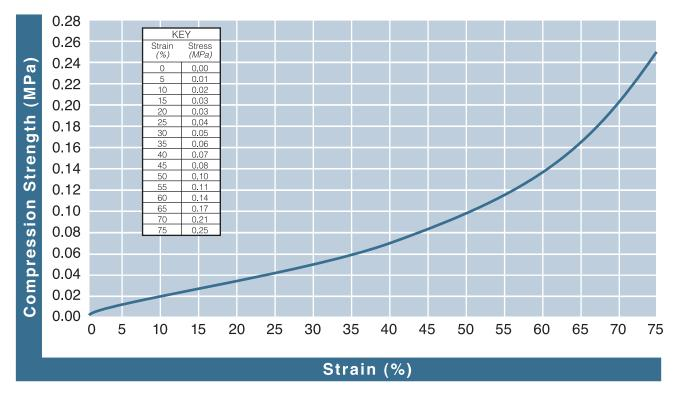
Note: 24 g/l = 1.5 pcf = 37.5 X (g/l = grams per liter; pcf = pounds per cubic foot; X = foam expansion ratio) 1 MPa = 1 N/mm<sup>2</sup> = 145.04 psi (Units of pressure/stress) Test Speed at 12.5 mm/minute (per ASTM-D3575)
