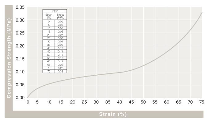
Note: 24 g/l = 1.5 pcf = 37X (g/l = grams per liter; pcf = pounds per cubic foot; X = foam expansion ratio) 1 MPa = 1 N/mm<sup>2</sup> = 145.04 psi (Units of pressure/stress) Test Speed at 12.5 mm/minute (per ASTM-D3575)
