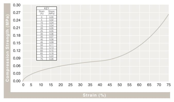
Note: 16 g/l = 1.0 pcf = 56X (g/l = grams per liter; pcf = pounds per cubic foot; X = foam expansion ratio) 1 MPa = 1 N/mm<sup>2</sup> = 145.04 psi (Units of pressure/stress) Test Speed at 12.5 mm/minute (per ASTM-D3575)
