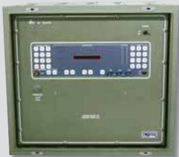
Customer-specific front panel with flexible skirt seal.
