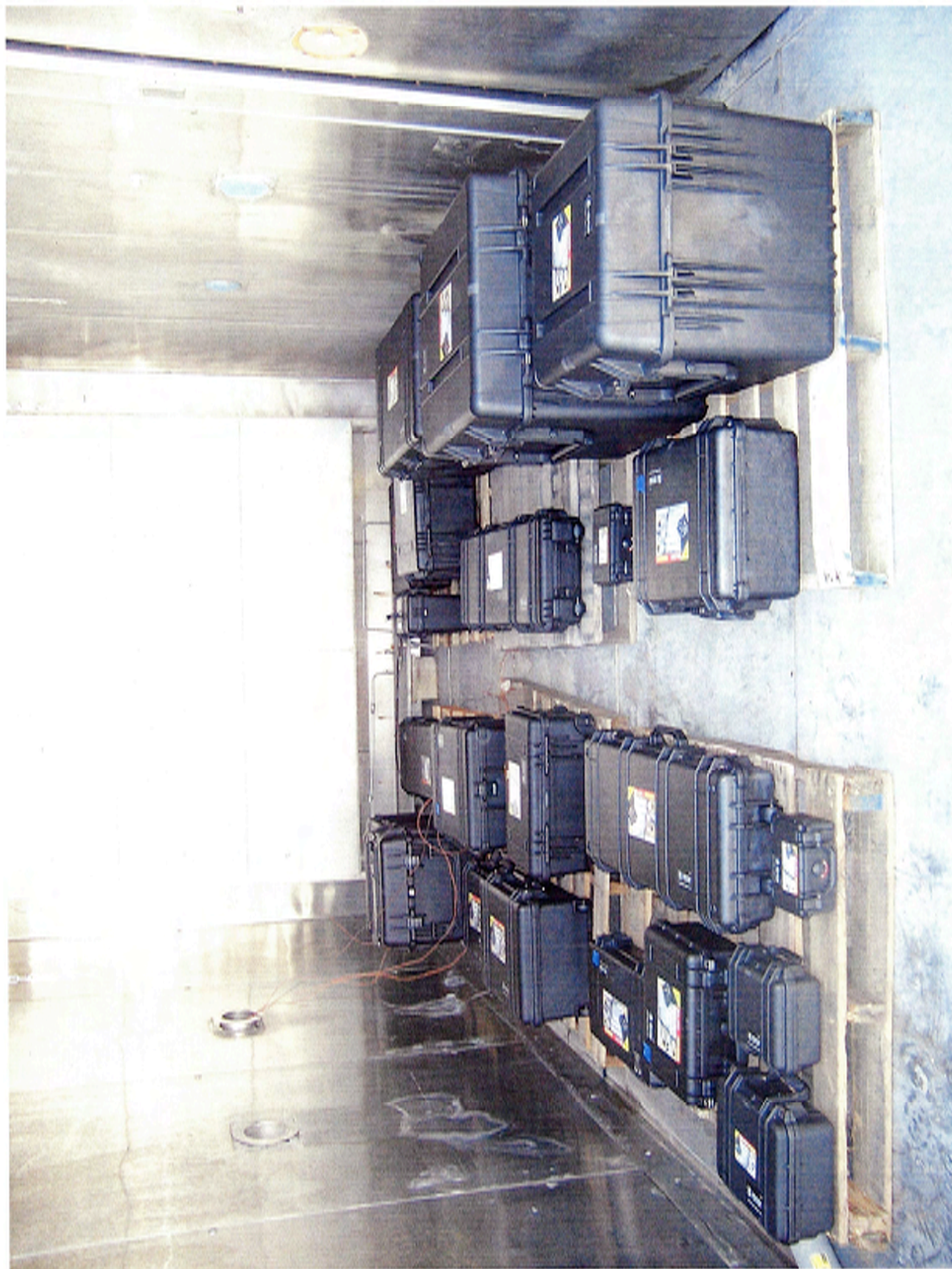
Photograph 6 Dry Heat Test Setup
