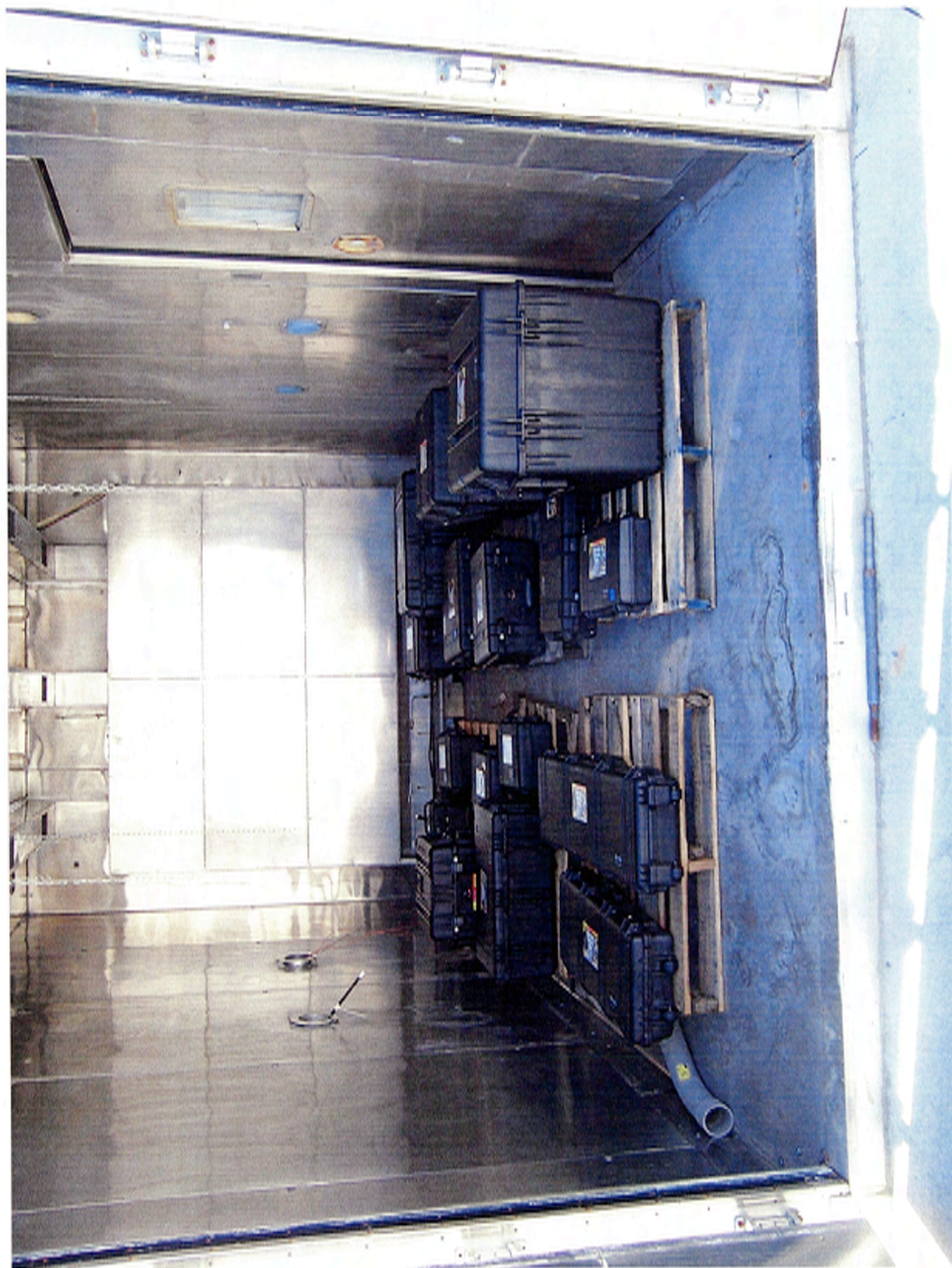
Photograph 1 Typical Pre-Conditioning Setup
